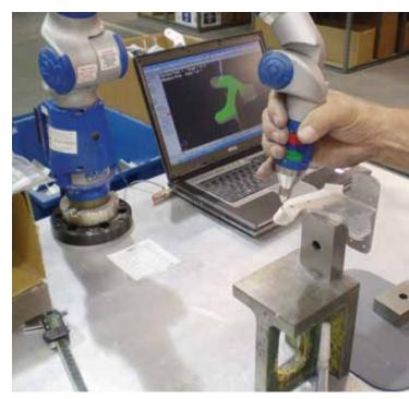
Parts are inspected against a solid model on the manufacturing floor.
